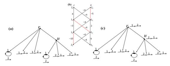
**Figure 10.** (a) Initial tree T and structures at its leaves. (b) Graph 2M and the matching P in it given in red. (c) Final reconstruction of structures for operation costs  $c_r = 1$  and  $c_s = 6$ : there are 3 cut events and 3 join events.
